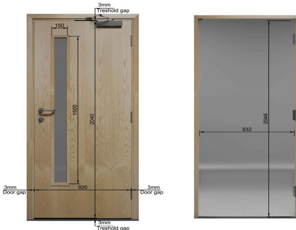
Figure 1: Dimensions of door and required door frame
