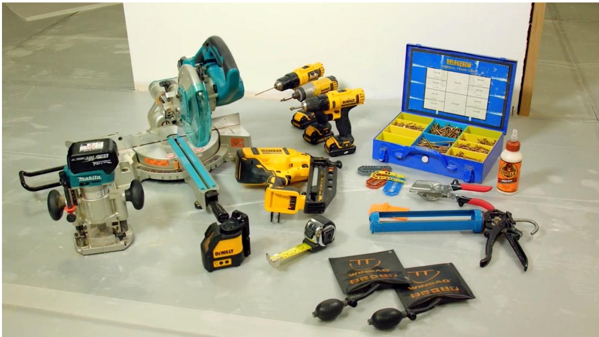
Figure 3: Section of tools required to fit a FD30 door.
