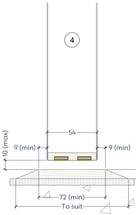
**Raised hardwood threshold: 640kg/m<sup>3</sup> (min)**
