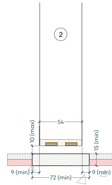
**Flush hardwood threshold: 640kg/m<sup>3</sup> (min):**
