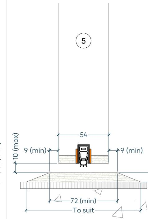
**Raised hardwood threshold: 640kg/m<sup>3</sup> (min)**
