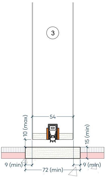
**Flush hardwood threshold: 640kg/m<sup>3</sup> (min)**
